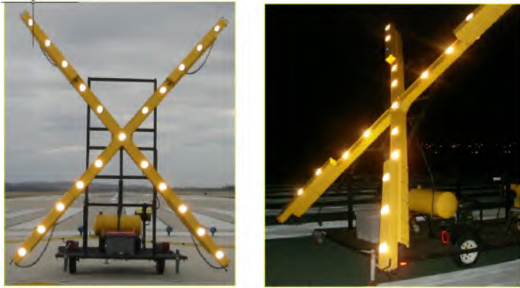
LIGHTED RUNWAY CLOSURE MARKER (PROVIDED BY CONTRACTOR)
